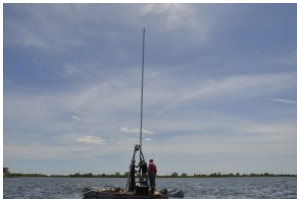
Scientists collect a sediment core from Salt Pond in Falmouth, Mass. The aluminum tube was vibrated into the muddy sediment at the bottom of the pond and then extracted with a hoist. The core provides evidence of intense storm events going back approximately 2,000 years.
